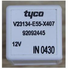
Unlike aerospace grade relays, which are typically hermetically sealed, automotive grade relays are at best environmentally sealed. So, de-lidding this device was a simple matter of using a small screw driver to pop off the cover. Once inside, the failure mode was obvious. The normally open contact set was badly pitted with obvious signs of material transfer from the movable contact to the stationary contact. The normally closed contact set, however, looked almost pristine.
